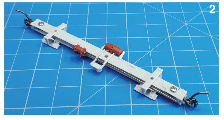
don't trust the glue joint between the weight material and resin so a styrene frame is built around the weight to ensure it doesn't rattle if it becomes lose. Keep the weight away from the truck screws so that the frame can be connected later to the tank.
