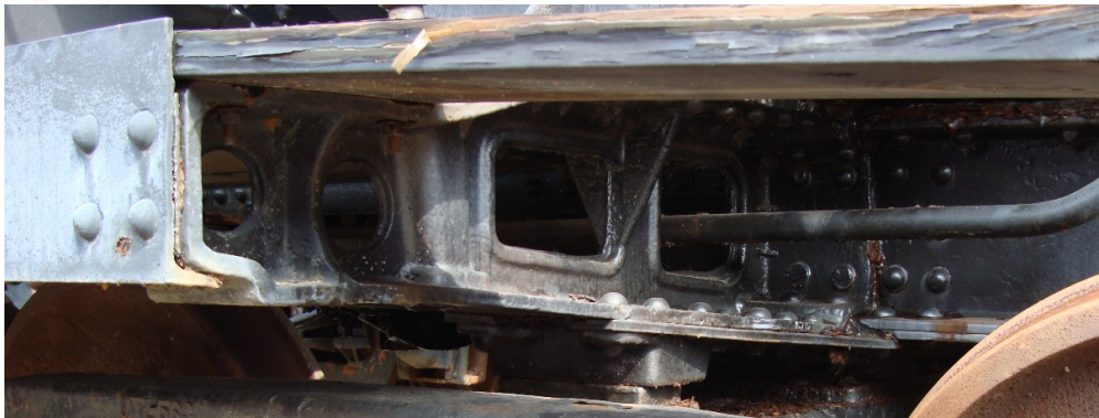
Photo of the more tapered, cast bolster on surviving 10000 gallon car UTLX 31589 at Galveston RR Museum. Photo courtesy of Morris Gold. Note the two extra holes under the running board and the tighter cluster of 4 rivets at the side sill.
