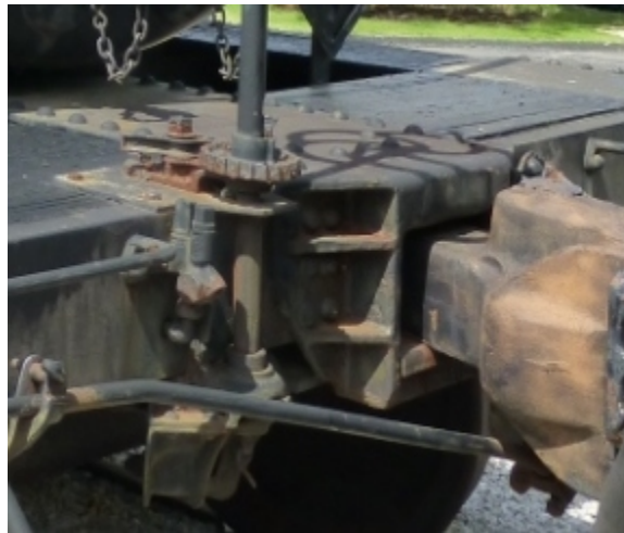
Another view of the brake wheel shaft outside the end sill on a late X-3 multi-compartment tank car at the National Museum of Transport in St. Louis, MO,
