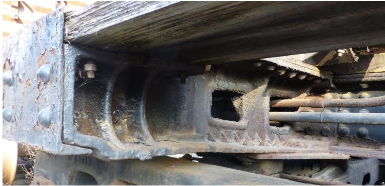
Photo of wider bolster casting on surviving example 6500 gallon car in Lake Superior RR Museum 2016.
