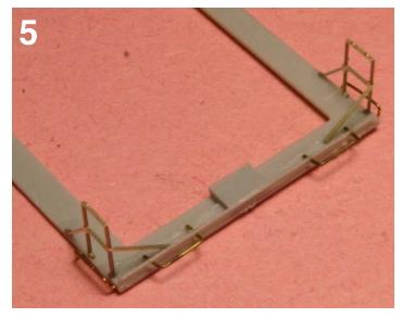
If necessary, the end sill pads and/or the tops of the draft gear can be filed so that the running board contacts the underframe at all six points without distortion or twisting. When satisfied, apply a little pressure to the underframe to set it down against the running board and apply CA to the six contact points. Be sure the running board is centered end to end and side to side.
