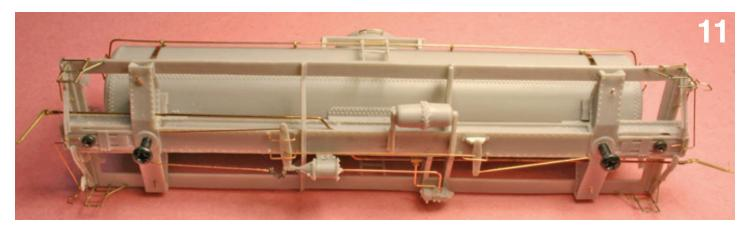
band is centered side to side on the tank. At one end wick AC into the wire hole from the bottom and bend the wire over against the underside of the bolster. Pull the other end tight to remove any slack in the band so that it is tight against the tank. When satisfied, repeat the process to secure that end. Trim off the excess from the wires, leaving just enough of the bent-over ends to keep the wires from pulling out of the bolster holes [Photos 7, 11].
