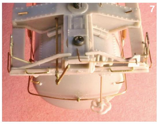
ervoir in addition to supporting the running board. These channels would extend from the center sill under its top flange out to the underside of the running board. The valve would sit on a plate spanning these channels above the reservoir. There were other variations to these conversions, so attention needs to be paid to the prototype in question. The Tangent Models three-compartment tank car has a Type 30 underframe and may serve as a guide, but note that it is a shorter 32-foot frame.
