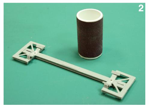
edges of this pad, making sure they are square. Clean and square off the edges of the end platform running boards so there will be a good joint for the long running boards between the platforms [Photo 1].
