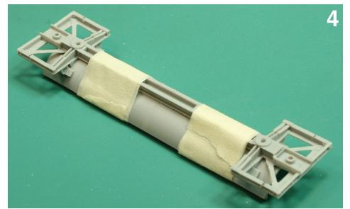
tom to the frame with small clamps or with a couple pieces of tape. Drill and tap couplers pockets and bolsters for 2-56 screws [Photos 3, 4].
