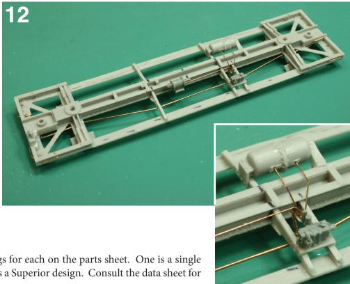
j. These cars had two types of geared handbrakes and there are castings for each on the parts sheet. One is a single piece that was an ACF design. The other is made up of two pieces and is a Superior design. Consult the data sheet for
