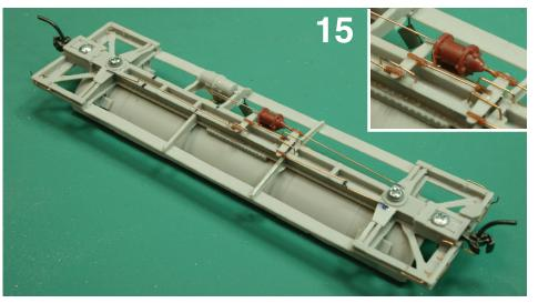
a piece of 0.020" wire centered on the brake lever hangers. There is no chain connected to the cylinder, as that's part of the brake housing.
