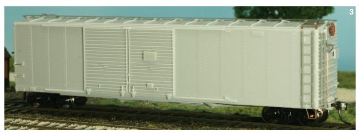
If you choose the Tichy ladders, an additional rung must be added. Trim the top of one ladder just above the bolts of the rung. Trim the bottom of another ladder just above the rung itself. Dress up the edges with a file to maintain spacing. Working on a plate of glass, cement the two sections together. There are small tabs on the underside of the Tichy ladder that need to be removed. Dress the ladder with a file, cut to fit, and attach to the car.
