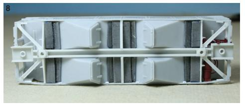
resin sill step form provided on the parts sheet. Trim the ends as necessary to fit in the form. Drill .020 inch holes in the sills to accept the steps and install them. If the sill castings are too narrow, the widths can be increased by attaching bits of styrene to the inside edges with ACC. Add the resin step braces between the steps and end sill. Attach pieces of .010 x .030 inch styrene inside each step to create the intermediate steps.
