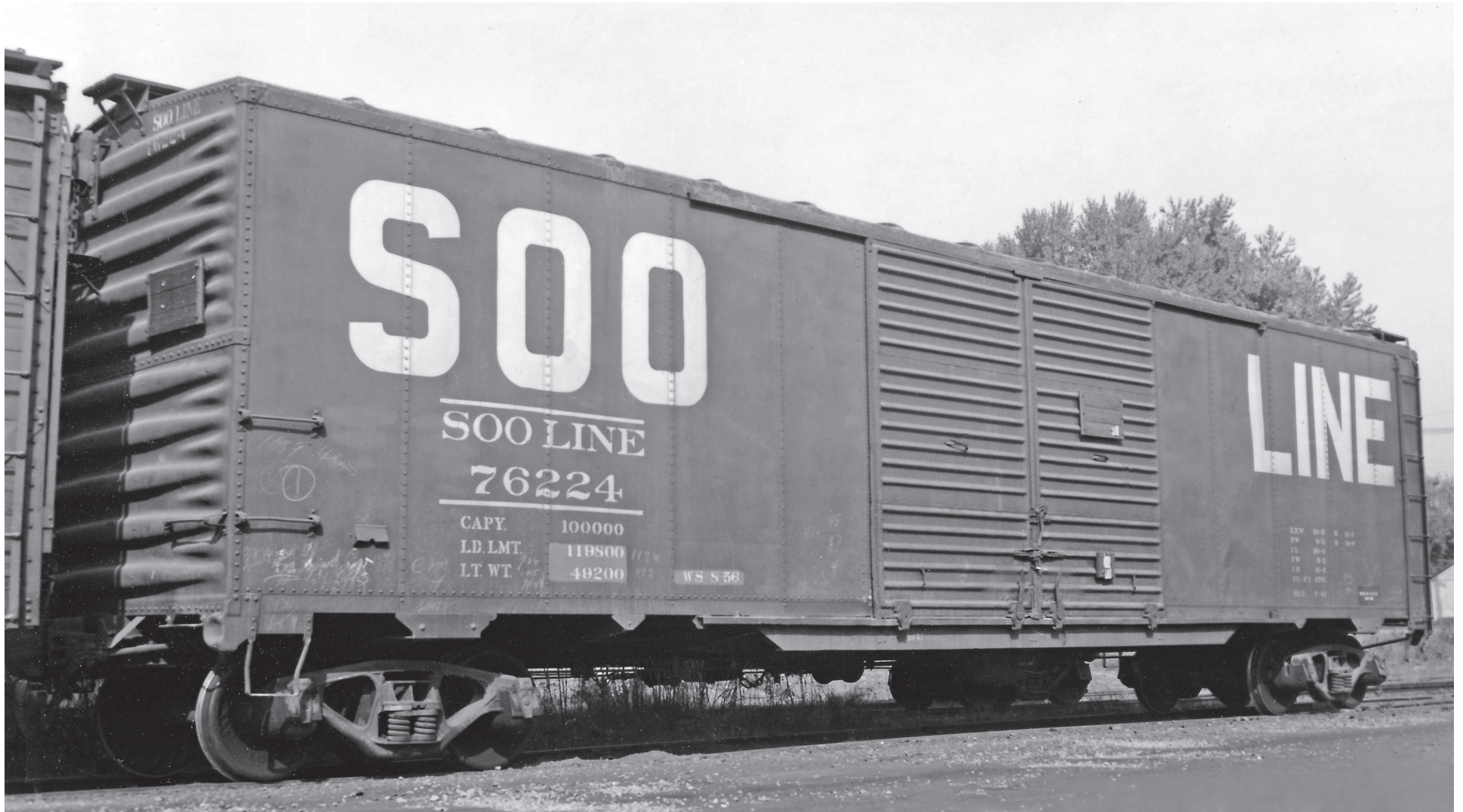
Car 76224 is from the 100-car series 76200-76398 (even) built by Pullman-Standard for the Soo Line in February 1942 (Lot 5689). Soo Line Railroad photo, Soo Line Historical and Technical Society Archives collection.
