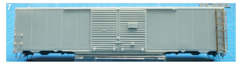
Attach coupler pockets to the underframe and drill and tap holes for 2-56 truck screws and 1-72 for coupler cover screws. The coupler boxes will accept only Kadee No. 158 semi-scale Whisker couplers.
