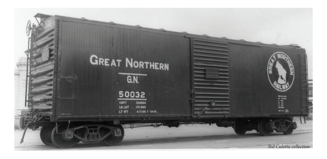
The first 1,000 cars of this design were constructed in 1937 by ACF and Pullman-Standard and were placed in the 50000 to 50999 series. The 1937 version was distinctive in its use of a two different types of vertical brake staffs and horizontal brake wheels. These were later replaced with standard power brake housings and cast wheels from various manufacturers.
