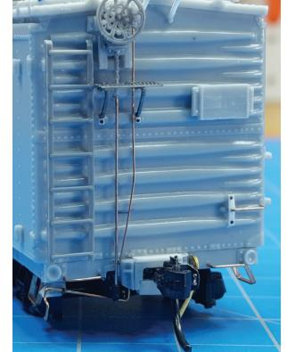
the end sill. Run 0.0125" wire from the end of the chain to the bell crank. Cement a small piece of scrap 0.030" x 0.040" styrene next to the brake housing mounting bracket. Cement the retainer valve to this bracket. Run a retainer valve line of 0.010" wire between the retainer and end sill.
