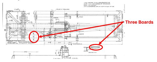
This can be modeled using 0.020" X 0.0125" styrene (not supplied in kit) as shown.
